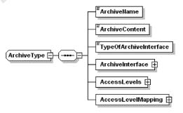
**Figure 12.15** The information stored locally at the archive profile allows for the automatic translation of system queries to a format that the custom content management application of the archive can parse, as well as for the translation of the response in the standardized data structures of the system
