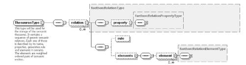
**Figure 12.5** The ThesaurusType. Initially only the rule and property fields are filled. In ontology update mode, the ontology update module uses them as input, together with the distinct semantic relations, in order to automatically generate the semantic views stored in the relation element fields
